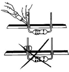
2. Make sure the solder joints are cone-shaped and shiny
