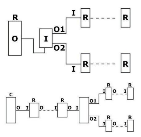
On the last device, the DMX cable has to be terminated with a terminator. Solder a 120  $\Omega$  resistor between signal (-) and signal (+) into a 3-pin XLR plug and connect it to the DMX output of the last fixture.
