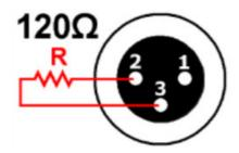
• Switch on the terminator on the splitter if you do not connect a device to the output.
