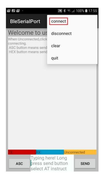
Make sure the Bluetooth® function is switched on and your phone is BLE compatible. You should now see the VMA338 under the name HMSoft. Connect to it.
