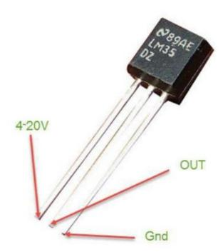
The LM35 is a common and easy-to-use temperature sensor. It does not require other hardware, you just need an analogue port to make it work. The difficulty lies in compiling the code to convert the analogue value it reads to Celsius temperature.
