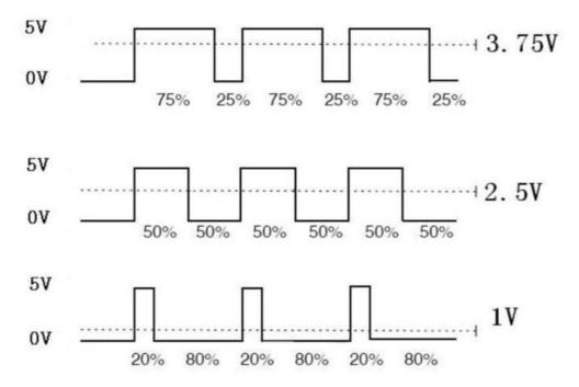
PWM has many applications: lamp brightness regulation, motor speed regulation, sound making, etc. The following are the basic parameters of PWM:
