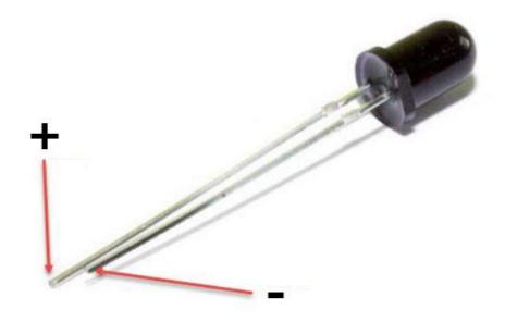
A flame sensor (IR receiving diode) is specifically used on robots to find the fire source. This sensor is highly sensitive to flames.
