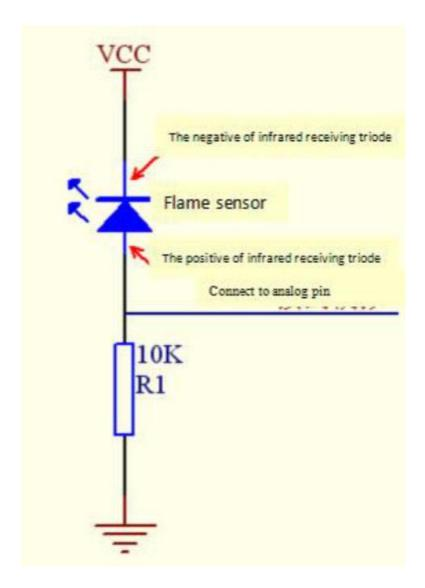
Connect the negative to the 5 V pin and the positive to the resistor. Connect the other end of the resistor to GND. Connect one end of a jumper wire to a clip, which is electrically connected to sensor positive, the other end to the analogue pin.
