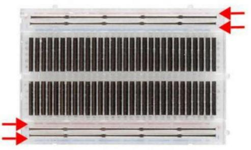
Chips have legs that come out of both sides and fit perfectly over the ravine. Since each leg on the IC is unique, we do not want both sides to be connected to each other. That is where the separation in the middle of the board comes in handy. Thus, we can connect components to each side of the IC without interfering with the functionality
