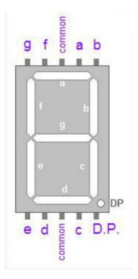
LED segment displays are common for displaying numerical information. They are widely applied on displays of ovens, washing machines, etc. the LED segment display is a semiconductor light-emitting device. Its basic unit is an LED (light-emitting diode). Segment displays can be divided into 7-segment and 8-segment displays.
