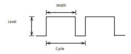
There are six PQM interfaces on Arduino ®, namely digital pin, 3, 5, 6, 9, 10 and 11. In this experiment, we will be using a potentiometer to control the LED brightness.
