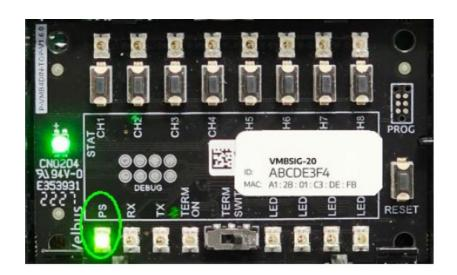
Press the RMT button (CH1) on the top left of the module.
