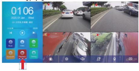
Tap the arrow in the diagram "playback" button View four-way surveillance video playback:
