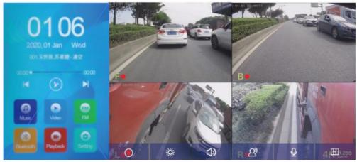
**Tap the arrow recording button to Start/Stop recording;** When there is a memory card inserted, there will be a memory card icon; The small red dots indicate that the video is being recorded.
