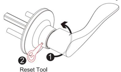
2. Press the Joint Point with the Reset Tool until it is fully depressed, then pull out the lever.
