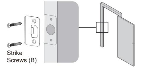
Note: The bevel of the Latch should be aligned with the bevel of the Strike.
