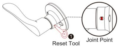
2. Press the Joint Point with the Reset Tool and pull out the lever simultaneously.
