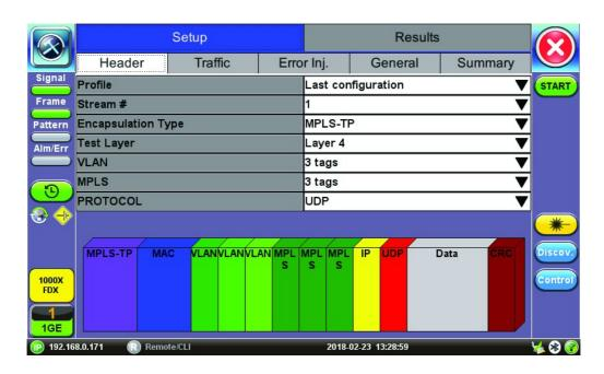
TCP Throughput Compliant with RFC 6349 Stateful TCP Test at line rate TCP Client and Server modes Compatible with iPerf Client/Server MTU search per RFC4821 Round Trip Time Measurement Configurable TCP Window sizes Multi-Window size tests
