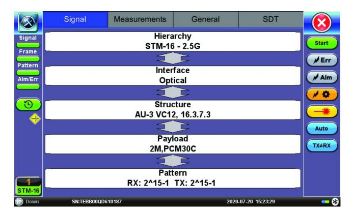
Test configuration, menus, and results are presented in VeEX's intuitive hierarchical test signal builder GUI, requiring little or no training for new or existing VePAL™ users, maintaining a consistent user experience from the lab to the field. Framed signals can be equipped with unstructured or structured payloads with selected test pattern filling the entire test payload (Bulk) or a structured payload (SDH/SONET framed client signal) with or without PDH/DSn multiplexed clients.
