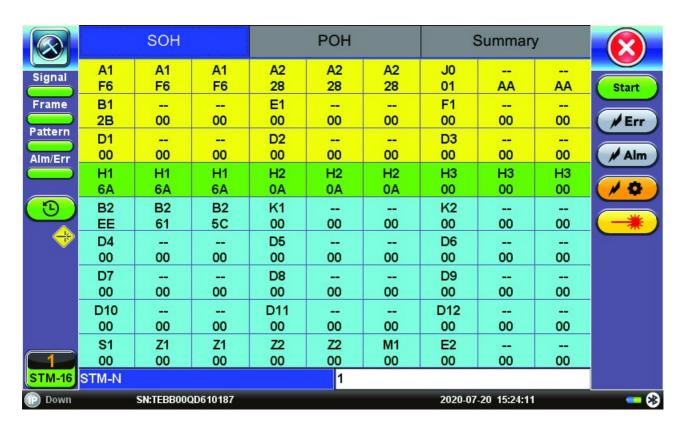
Overhead byte control allows the manipulation and easy encoding of transmitted overhead bytes in both terminated and payload through modes to stress the network responses to various conditions.
