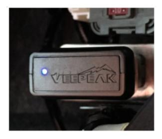
Step 2: Install Device Plug in the device. Turn on car ignition.
