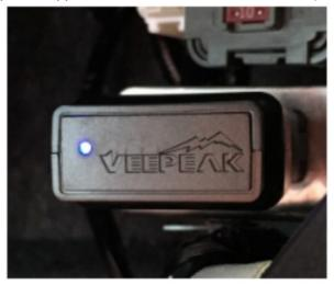
Step 2: Install Device Plug in the device. Turn on car rogation.
