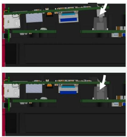
10. Check the correct position of the EMC spring after assembly.
