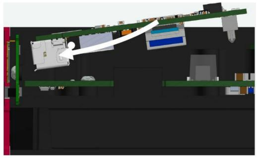
9. Carefully connect the rear connector of the module to the main board connector. Insert the module as vertically as possible.
