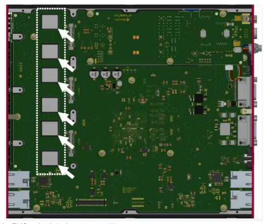
2. Check that the EMC spring is in the correct position.
