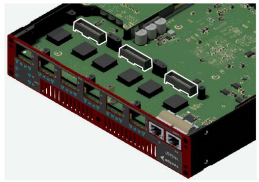
7. Hold the module over the corresponding slot on the main board.
