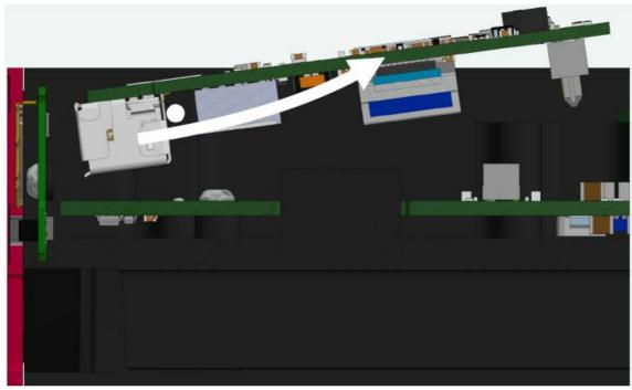
7. The module can then be removed from the housing.
