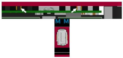
11. Tighten all screws (5) of each replaced module with a Torx TX 8 screwdriver to a torque of 0.5 Nm.
