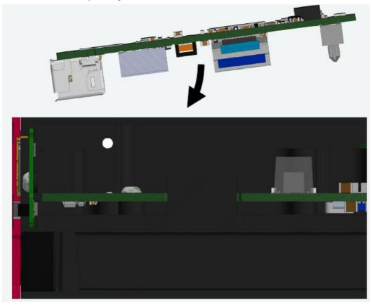
8. Slide the module towards the front panel and through its openings until the connectors are flush with the outside of the front panel.
