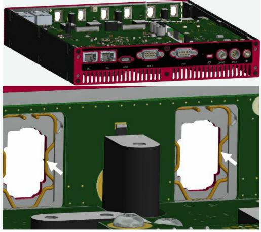
3. Unpack the replacement module. Remove the protective film from the gap pads. Do not remove the gap pads from the heat sink!
