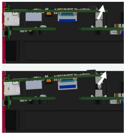
6. Pull the module inwards until the front connector of the module is completely pulled through the LED board.
