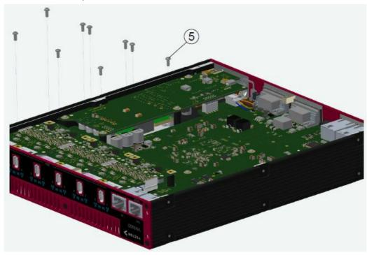
5. Lift up on the back of the module until it is disconnected from the connector on the main board.
