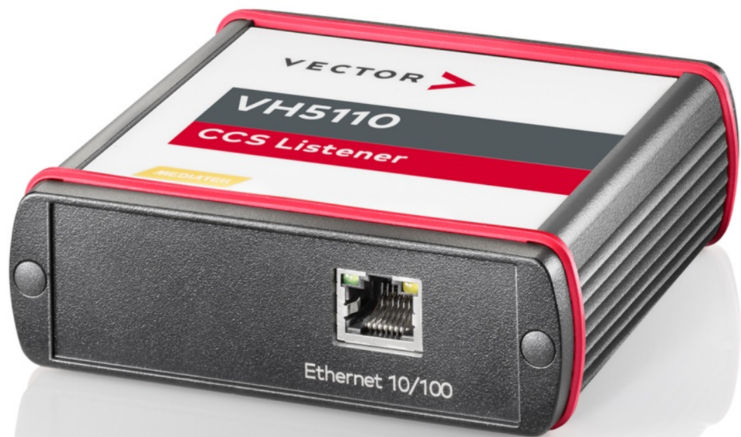
Figure 1: VH5110 with RJ45 Ethernet connector With the RJ45 Ethernet connector, the VH5110 will be connected to the computer where CANoe is running. For this purpose a separate Ethernet adapter (e.g. Vector VN5610A) is necessary. Also, the built-in Ethernet adapter of the computer can be used. The VH5110 can also be used for logging of the charging communication. In this case, the VH5110 will be directly connected to the Ethernet port of a suitable data logger. The CANoe is then only used for later offline analysis. The LEDs on the RJ45 socket indicate the following status:
