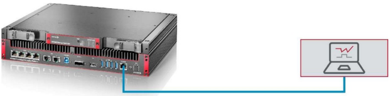
Figure 4: Connecting VP7400 to configuration computer
