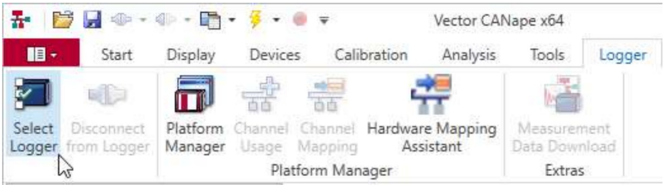
Figure 9: Logger ribbon in Vector CANape
