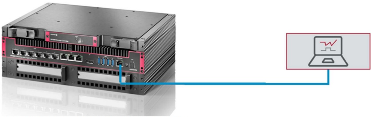
Figure 5: Connecting VP7500 to configuration computer
