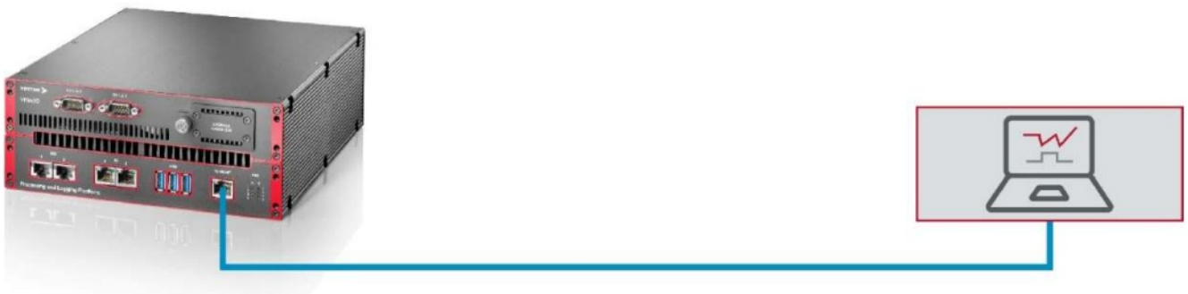
Figure 3: Connecting VP6400 to configuration computer
