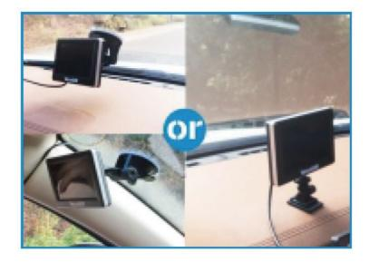
Attach the monitor to the dashboard or to the head-liner using sticker bracket or suction bracket. Attach monitor to mount, and adjust mounting angle to allow optimum driver viewing comfort.
