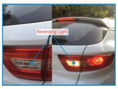
2. Find the position of the car's reversing light, then remove the interior baffle near the rear of the trunk and find the line position of the reversing light (It's recommended to use the electroscope to detect the positive and negative poles of the reversing line).
