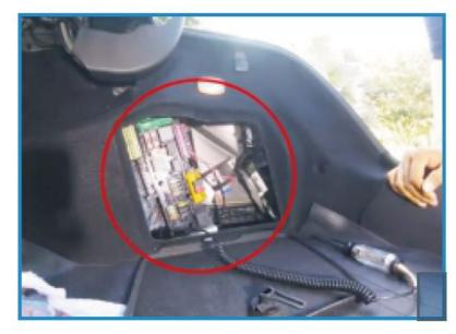
3. Remove the license plate and put the extension cable of the camera through the hole(You will need to drill a hole if necessary )on the back of the license plate on trunk, and connect the camera power cable to the camera extension cable, tape the connector together.
