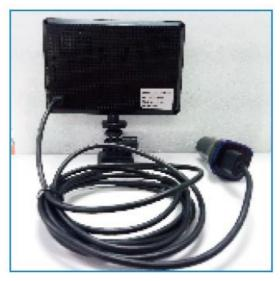
6. Connect the car cigarette lighter to the USB cable, then connect the monitor (If without a car cigarette lighter, you can put the USB cable into the car's USB port directly).
