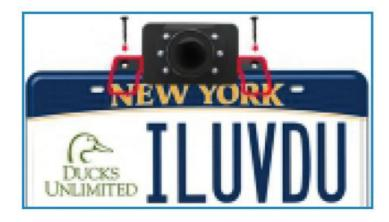
If you worry about that the camera is not secure enough, you can use the self-tapping screws to fix the camera on the car.
