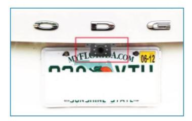
This wireless camera must rely on the license plate to be fixed. Please do not install the camera elsewhere in the car.
