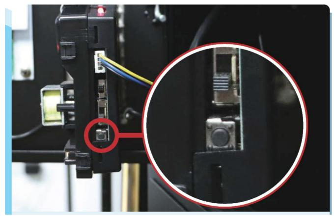
2. The indicator light will start flashing to indicate that it is in the settings mode.
