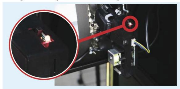
3. Insert coins one by one until the indicator light is no longer flashing. You will hear a beep indicating setup is complete.
