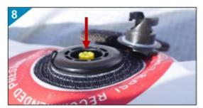
• To deflate, press and turn the yellow valve stem 90° to the lower position.
