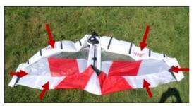
Fold the leading and trailing edge toward each other and roll up the wing from the wingtips before placing it in the extended bag.
