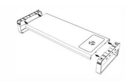
Take out the support components from the packing box, insert them into the aluminum alloy panel guide as the figure above, keep it firm and steady, then it can be put on the desk and used.
