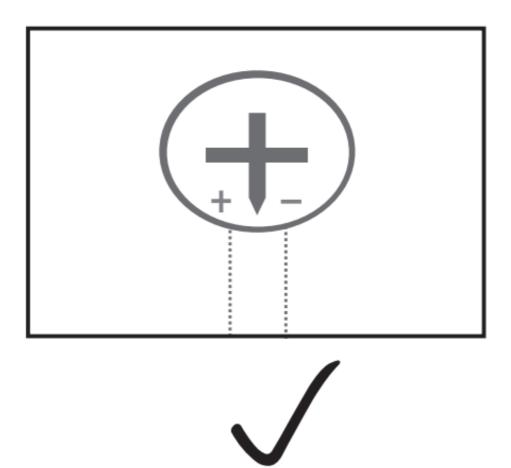
Insert bolt when connecting piece direction is properly lined up.
