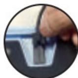
Align the notch of the anti-shedding sheath downwards with the Type-C wire
