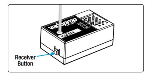
The S2R comes with failsafe set to neutral position on steering and throttle channel. In the event of loss of signal the motor will stop and the vehicle will drift. If the signal is regained normal function will return. If you wish to program the failsafe to a custom setting just follow these simple steps:
