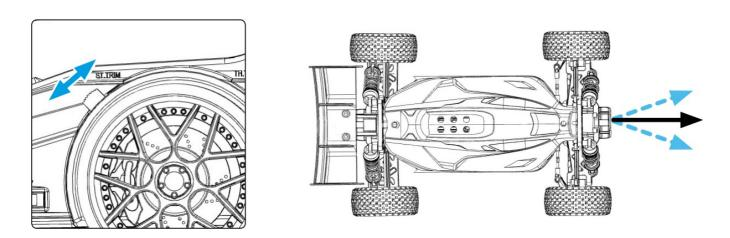
The steering trim is used to adjust the steering setting so that the car moves in a straight line without using the steering wheel to compensate.
