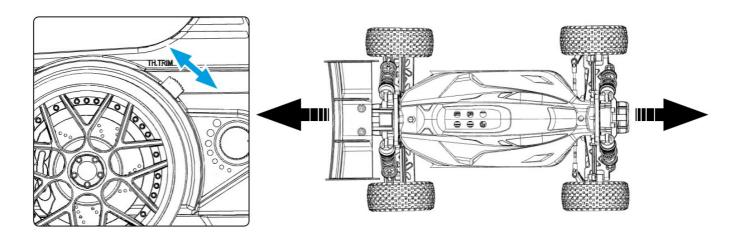
The throttle trim is used to adjust the setting of the neutral position of the throttle without using the throttle/brake trigger to
