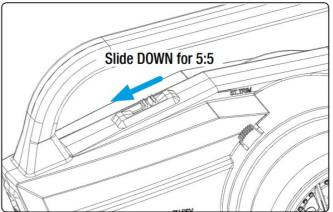
Adjust the proportion of throttle signal on either side of the center trigger position.
