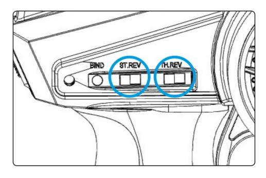
TH.REV (Steering Reverse): This function reverses the rotation direction of the THROTTLE servo.
