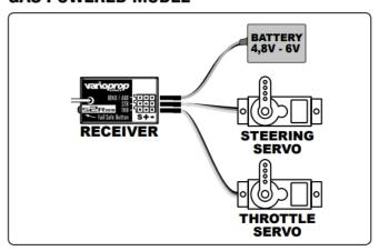
Install the Receiver in your model using double-sided Velcro. Velcro will hold the receiver in place and protect it from vibrations. Mount the antenna up and away from the vehicle in an antenna tube. The higher up the antenna is, the better signal it will receive. Install and connect the receiver, servos and other components in accordance with the "Assembly Precautions".
