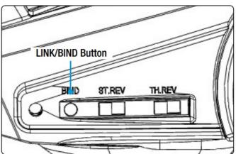
Each transmitter has an individually assigned, unique ID code. In order to start operation, the receiver must be linked with the ID code of the transmitter with which it is being paired. Once the link is made, the ID code is stored in the receiver and no further linking is necessary unless the receiver needs to be used with another Varioprop S2R transmitter.
