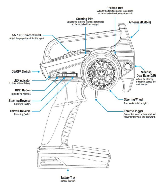
**WARNING**: Do not cover/hold the built-in antenna part of the transmitter by your hand during running. Do not put any conductive plate/sticker on the antenna part. Otherwise, the operating range may become shorter.
