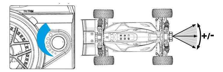
Use this function to adjust the steering travel of your model. If the model understeers while cornering, add steering by
