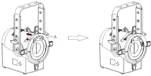
• Step 2. Snap the iris into the luminaire as shown.
