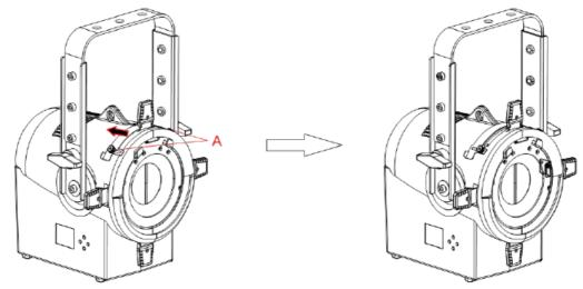
• Step 2. Snap the gobo holder into the luminaire.
