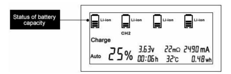
If multiple batteries are placed in the charger at the same time, we press the DISPLAY button several times to display the battery data of each slot in turn.each slot is independent of the other, there are slots to charge, there are slots to discharge, there are slots to repair the process, without interference with each other. If CH1 is displayed, it will be the data of the first slot battery.
