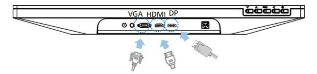
The DP port is exclusive for TMC215 & TMC270. The display cable shall vary with the display interface, and adapter connectors are sometimes needed.
