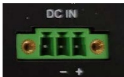
Figure 5-1-1 DC24V power input connector
