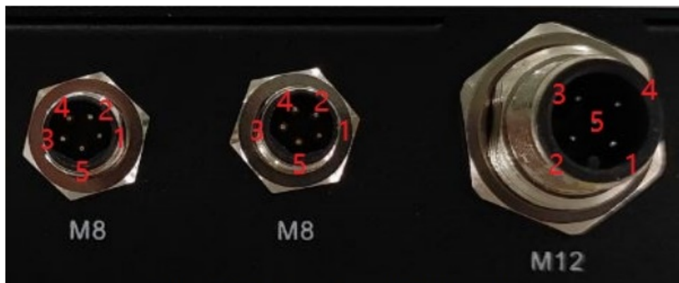
Figure 5-2-1 Power Output & CAN Interface
