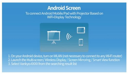
**Step 3:** Activate Multi-screen/ Wireless display/ Smart View function on your Android device and search for the projector.
