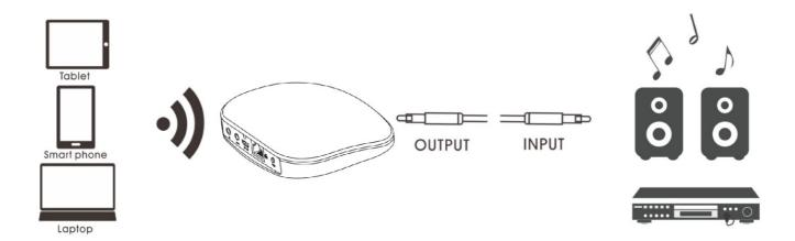
The PASTREAM Receiver is a device that receives internet streaming music or other wireless music from any wifi enabled device. Multiple PASTREAM receivers can be used in a single distributed audio system to create multiple streaming sources.
