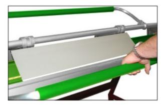
C. Rotate the front hinge up to flatten the angle against F-Bar to complete the hem. Note: It is recommended that you make practice bends with scrap until satisfied with the results.
