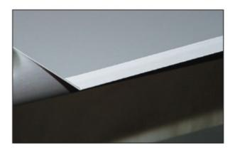
D. Standard Hem. Hems can be formed on all Mark Series™ brakes, TrimMaster® brakes, and Metal Master® 20 brakes. Visit <a href="https://www.van-mark.com">www.van-mark.com</a> for more tips and ideas.
