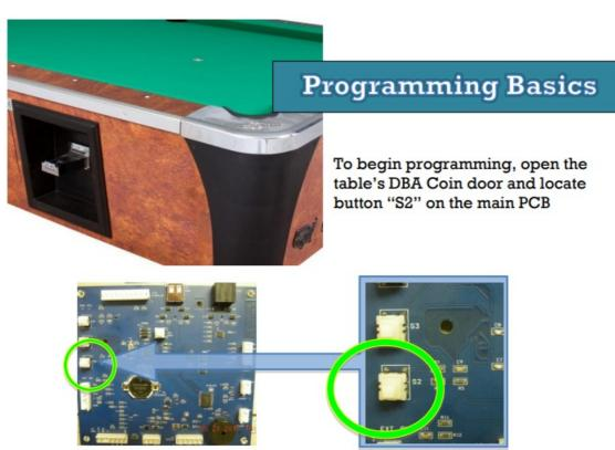
• To go into program mode hold down the S2 switch as the display counts down from 5, release after your display shows
