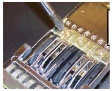
6. Remove the Phillips screw or screws holding the insert retainer plate and you will have access to all the inserts.
