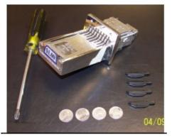
2. To gain access to the inserts, put your coins into the correct slots and then push in the handle.
