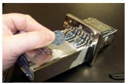
3. After pushing in the chute and your coins drop out, you can now access the inserts and a section that may contain spare inserts. Continue to hold the handle in as shown...
