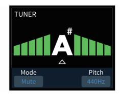
Quick access knob 3 adjusts the pitch calibration (REF PITCH), ranging from 435Hz to 445Hz. Standard pitch is set at 440Hz. Quick access knob 1 lets you select the tuner mode from Bypass (for dry signal through), Thru (for eect signal through) or Mute (for silent tuning). You can exit the tuner either by pressing any footswitch or by pressing the EXIT button.
