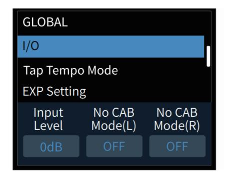
No CAB Mode is for connecting to instrument amplifiers without changing saved presets. Turning this on will bypass the CAB module for GP-100's L/R output channels ignoring preset settings. You can apply different settings on L/R output channels for different scenarios. Default is set to OFF.
