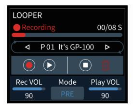
**NOTE:** You can exit the LOOPER by pressing the EXIT button. The function of the footswitches in this interface, tap footswitch [-] to record / play/ overdub, tap footswitch [+] to stop, hold to clear. Simultaneously hold two footswitch's to exit.
