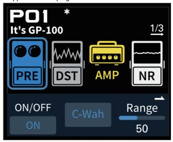
Some effects have several parameters, but only three parameters appear per page. Press the PARA knob button to turn the page to view the other available parameters.
