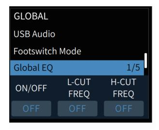
Global EQ contains Low Cut / High Cut, and 4 bands of parametric EQ. Every frequency band can be freely adjusted based on your needs. There are total 6 of them.
