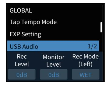
This menu is to set up USB audio settings when using GP- 100 as a USB audio interface.
