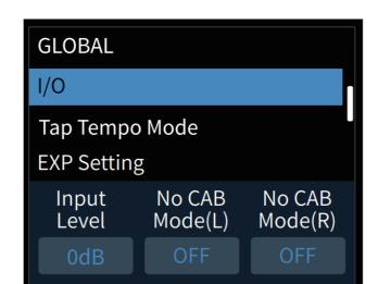
Turn the PARA knob to select settings in the GLOBAL menu. You can use the three Quick adjust knobs to adjust the parameters directly above the knobs. A page number will appear at the top right of the screen. Press the PARA knob button to turn the page to view the other available parameters.
