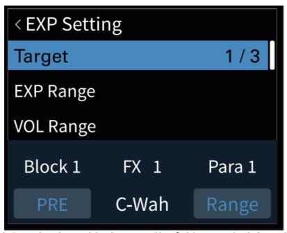
Use Quick access knob 1 to select the module placement. Use Quick access knob 3 to select the effects parameter. Press the PARA button to flip through the panel. You can also turn the expression pedal off by selecting OFF in the settings panel.
