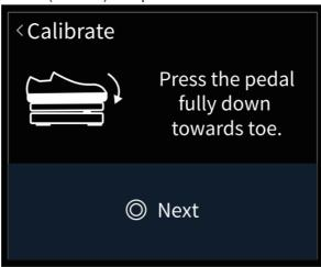
Then, press the pedal toe down strongly and press the PARA button to next step.
