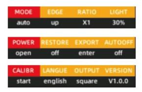
Press the MENU key in oscilloscope mode to enter or exit menu mode; In menu mode, press the arrow keys left and right to select menu items, and press the arrow keys up and down to adjust the settings.
