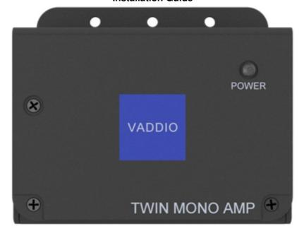
The Twin Mono AMP is an 8-ohm, 30-watt mono-power audio amplifier with a single differential input feeding two amplified outputs, each capable of driving into loads as low as 4 ohms. The Twin Mono AMP drives two analog speakers such as the Vaddio Ceiling Speaker, EasyTalk Sound Bar, or third-party speakers.
