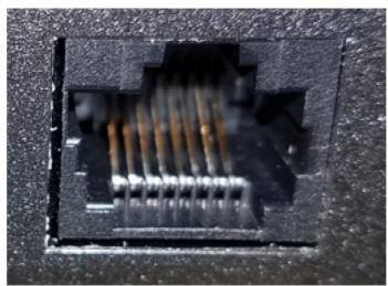
Damaged – Bent contact fingers will NOT make reliable contact with cable connector
