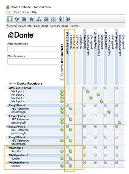
4. Select the box where each Dante receiver device intersects with the Mix Output 1 channel.
