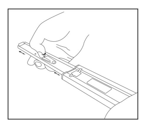
**Step 2** Installation Instruction Make sure the slides are leveled during the installation process.
