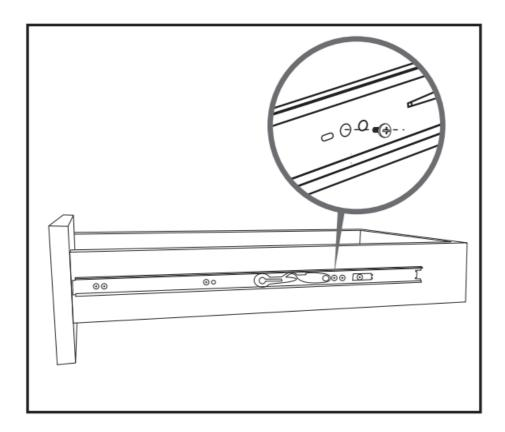
Step 6 Move the metal retainer to the front of cabinet member and insert the drawer box carefully.
