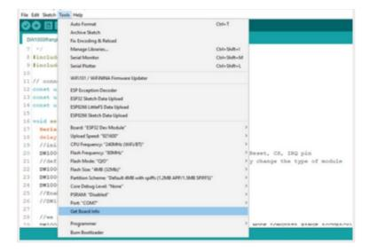
Also, make sure to select the correct COM port, which you can find in the Device Manager. Your ESP32 Ultra Wideband board is now set up for serial communication.
