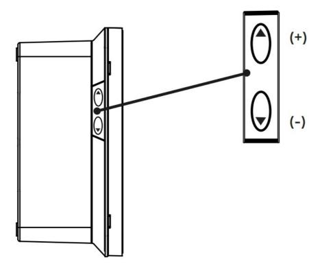
To access the configuration you must press the two buttons simultaneously for 4 to 5 seconds. for 4 or 5 seconds.
