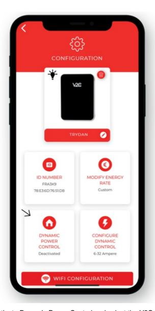
4. Activate Dynamic Power Control and select the V2C 2.0 meter and installation type.
