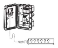
2. Locate the phase supplying the whole installation and connect the clamp meter. Release the sensor and fit around the power cable. Close the clip to hold it firmly in place. Normally, this is the connection from the meter, which is grey, black or brown. If it is a three-phase installation, you must use the 3 clamps (view slave graphic) and must all previously exposed cables. **IMPORTANT**: the clip should cover the ENTIRE phase to read the energy of the whole installation (house + e-Charger).
