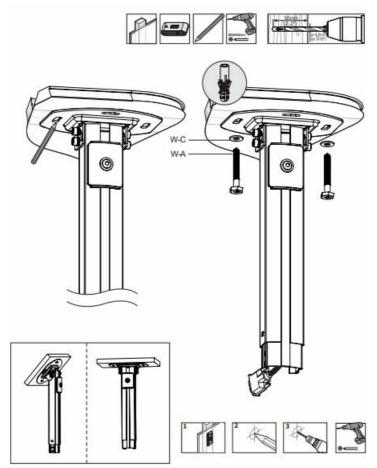
• OPTION B: Concrete/Brick Mounting Use the top plate of the arm (A) to mark mounting holes on the ceiling. Using a %" drill bit, drill approximately 2.4" into the ceiling. Use concrete anchors (W-B), bolts (W-A), and washers (W-C) to mount the arm (A) as shown in the diagram.
