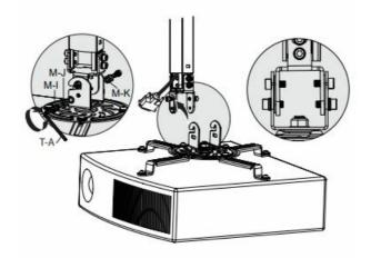
• Adjust height and tilt of mount using the allen wrench (T-A).
