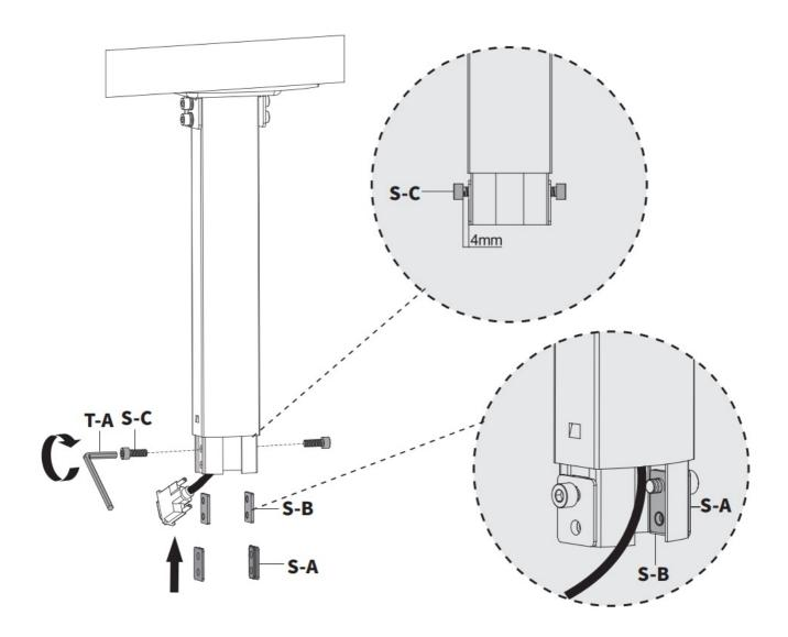
Latch Shelf (B) onto previous installed screws and install remaining M5x12mm Screws (S-C) in remaining set of holes. Secure all screws with 4mm Allen Wrench )T-A).
