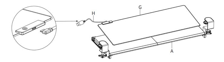
• Place Mouse Pad (G) on Keyboard Tray (A). Plug Power Cable (H) into Mouse Pad (G) and plug the other end into a 5V USB power supply.
