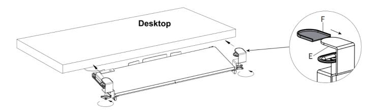
• Place Pads (F) on the underside of each Clamp (E). Place assembled keyboard mount on the edge of the desktop and tighten Clamps (E).
