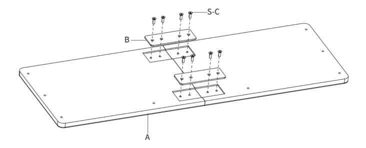
• Assemble Keyboard Tray (A) using Connecting Plates (B) and M5x12mm Flat Head Screws (S-C). Tighten with a Phillips screwdriver..
