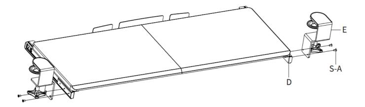
• Assemble Clamps (E) to the Slider Brackets (D) using M4x7mm Flat Head Screws (S-A). Tighten with a Phillips screwdriver.
