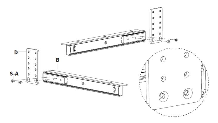
**NOTE:** Countersunk holes should be facing outward.
