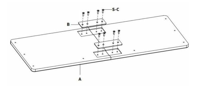
Attach the Keyboard Stop (C) to the back of the Keyboard Tray (A) using M5x12 Flat Head Screws (S-C). Tighten with a Phillips screwdriver.
