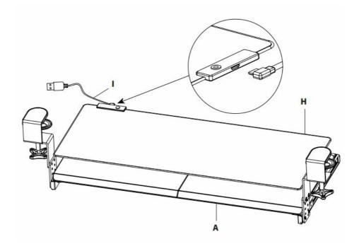
To ensure the keyboard tray assembly is level, do not over-tighten Clamps (F). Slide Keyboard Tray (A) forward/back to the desired position.
