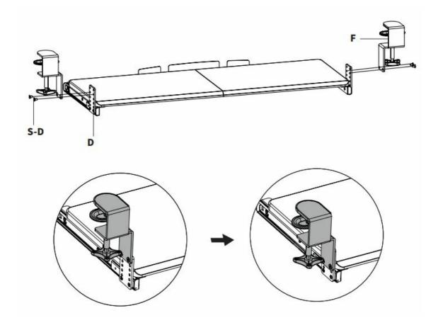
**STEP 6**Place Pads (G) on the underside of each Clamp (F). Place assembled keyboard mount on the edge of the desktop and tighten Clamps (F).
