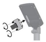
2. Labels indicating the pad to be connected are attached to the cable. Connect the cable to the OUTPUT jack of each pad as shown in the illustration.
