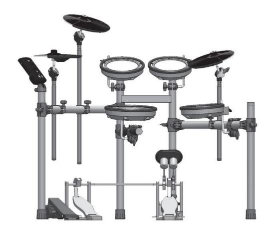
Position the two beaters equally apart from the center of the pad as shown in the figure at left. If one of the beater is further away from the center than the other, the sound from the further beater will be lower in volume, or will not sound as desired.
