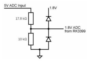
It is safe to connect A0, A3 or A4 channel to any pin in the 40-pin GPIO header, because they can measure voltage up to 5V. If you want to measure voltage higher than 5V, you will need to implement an additional voltage divider.
