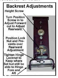
A driver's backrest that becomes part of your seat. No bars in the way of the driver's hips and legs or passenger's legs. Folds forward to ease passenger getting on or off and adds to safety by getting out of the way in sudden stops. Has up and down height adjustments, as well as driver seating position, back and forth, to help driver sit upright to avoid slouching, a big factor in driver fatigue. Included is our Quickest, that allows you to pull up on Backrest to remove.
