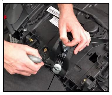
**Step 5** Line up Hole in Mounting Bracket with Hole on bike. Insert Bolt with Lock Washer and Fender Washer, through hole into threaded hole in Mounting Bracket and tighten snuggly, but do not over tighten. Tighten Bolts in Step 2. Finally, Slide Utopia Upright with Utopia Driver Backrest into slit in seat
