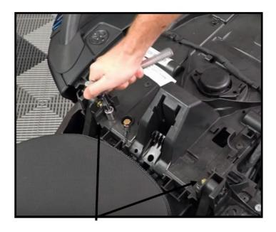
Step 2 Loosen the 2 bolts on the Seat Tray, with 13mm socket, back 2 full turns, or so, but not all the way out.
