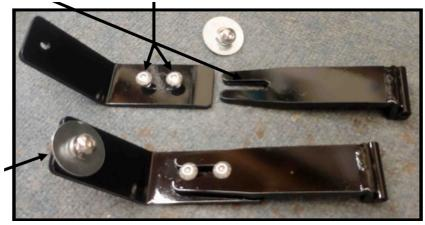
**Step 4** Insert Utopia Mounting Bracket into receiver slot, as far as you can, on top of the 1" Square Bar under Seat Tray. With some force push back, or hit top of Mounting Brick -et popping it in place on top of the 1" Square Bar.
