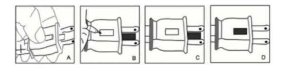
To prevent risk of fire, do not replace attachment plug. Contains a safety device (fuse)that should not be removed. Discard product if the attachment plug is damaged.
