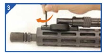
4. ~ 4. Pay special attention that the T-Nut catches on the slot and rotates the T-Nut to a 90 degree perpendicular ali9nment in relation to the slot . This can often be seen within the first 1 /4" tum of the screw if the T-Nut Gap was adjusted properly earlier on.
