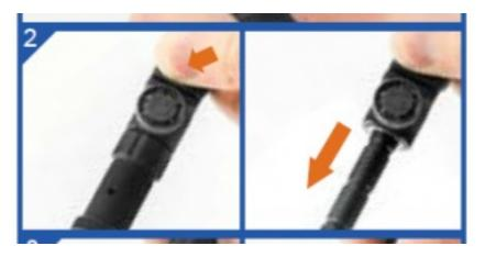
3. At full extension, press the tab once while simultaneously pushing the leg extension back in to traverse through the shorter, lengths. The notches in the leg extension will lock with the tab each time you reach, a preset length. Lock the thumb wheel of each bipod leg by turning clockwise until tightened once the desired center height is achieved.
