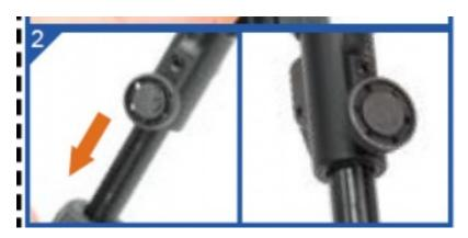
3. To retract the bipod leg, loosen the Locking Thumb Wheel first. Press down the Leg Retraction Clamp before you push the extended leg upward into the housing.
