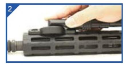
3. Once seated and the "biased", hold the mounting base in place and retighten the T-Nuts by turning the Allen Wreanch clockwise until securely tightened. Recommended torque value: 35in-lbs.
