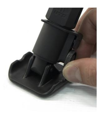
2. Pull down the footpad to Increase the length of the leg extension. Note that the leg extension is under spring tension as it is designed to automatically retract. The leg extension is keyed and once at the desired length Is secured in place by turning back the locking thumbwheel clockwise until it stops.
