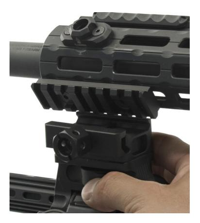
3. Retighten the side locking plate nut by turning it clockwise until snug or to 501n-lb using a torque wrench equipped with a 5/8" socket.
