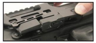
2. Press and hold down the spring-loaded side plate and locking tab located at the bottom center of the mount to allow clearance for the adjustment gear to rotate.
