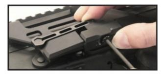
4. Once proper tension is achieved, release the spring-loaded side plate and locking tab ensuring the gear returns to its keyed position.
