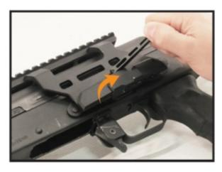
4. Proper mount retention is achieved when the mount attaches securely to the receiver side rail without any movement forward, rearward, up, or down with the lever in its locked position.
