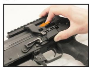
3. Turn the quick release lever completely back to the right to its locked position and test mount tension. If tension is too loose or too tight and you cannot turn the lever completely to the locked position proceed to "Adjusting Mount Tension" instructions.
