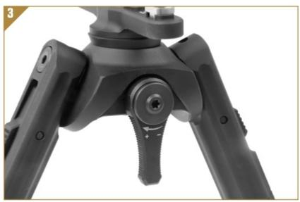
With max tension achieved, reinstall the lever with it pointing straight down. Using the T15 Torx wrench, reinstall the lever cap and screw. Recommended torque value is 15in-lbs.
