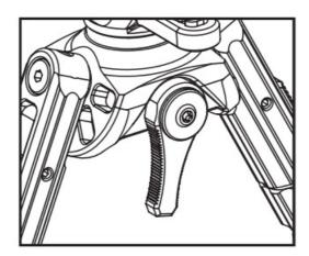
The RECON 360° TL features a tension adjustment lever that controls the felt resistance or tension that is applied when panning and tilting. The tension adjustment range and the distance the lever must be thrown is user configurable.
